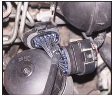
Rapid Power Connectors Plugged in
