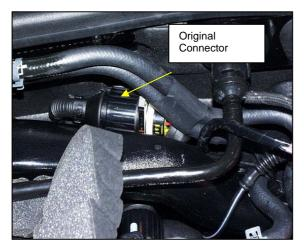
+12 V +12 V Battery Ground connection The construction of all injector pump engines is similar. The first picture is showing an example of a Volkswagen Passat 1.9tdi (engine is mounted longitudinal). Dismount the big round connector on the back side from the cylinder head.
