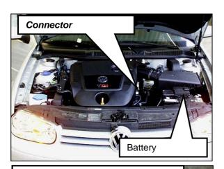
Disonnect original connector and placePower unit loom between them.
