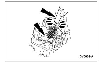
4. Install new O-rings on the fuel injector. Lubricate the fuel injector and O-rings liberally with clean engine oil.
