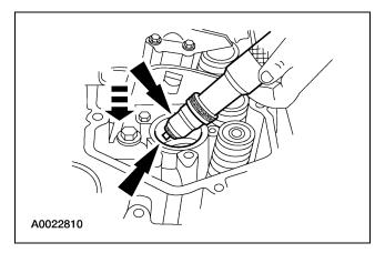
3. Clean the fuel injector sleeve and bore, using the fuel injector sleeve brush. Remove any sealant residue from the fuel injector bore.
