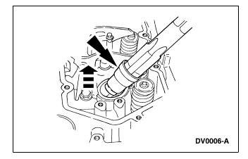
11. Remove sealant residue and all foreign material from the cylinder head fuel injector bore, using the injector sleeve brush.
