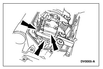
7. Place the fuel injector into the injector protective sleeve.
