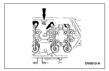
4. **NOTE:** Rocker arm removed for clarity. Remove the bolt and the oil deflector from the fuel injector hold-down plate.
