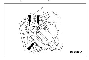
5. Remove the fuel injector outboard retaining bolts.
