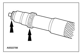
2. Position the fuel injector sleeve into the cylinder head fuel injector bore. Seat the fuel injector sleeve in the fuel injector bore, using a rubber mallet. Remove Injector Sleeve Replacer tool from the cylinder head fuel injector bore.
