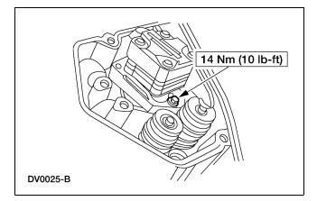
8. Install the oil deflector on the fuel injector hold-down plate.
