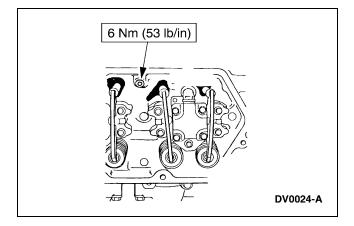
10. Tighten the fuel drain plug located at the rear of each cylinder head.
