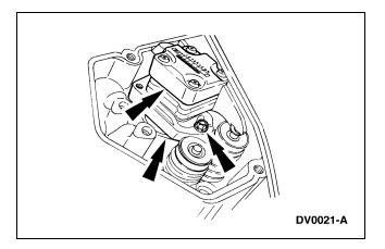
6. **NOTE:** When removing the fuel injectors, it is important that all three injector O-rings and the injector tip copper washer are removed from the injector bore. If the copper washer is not on the injector when removed from the cylinder head, make sure to remove it from the injector bore.
