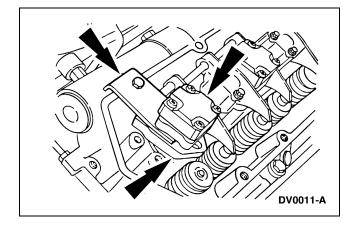
7. Install the fuel injector outboard retaining bolts.
