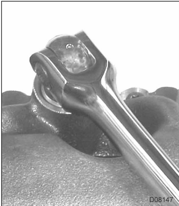
Figure 4 Removing Crankcase-to-Head Tube Plug (square head socket shown)
