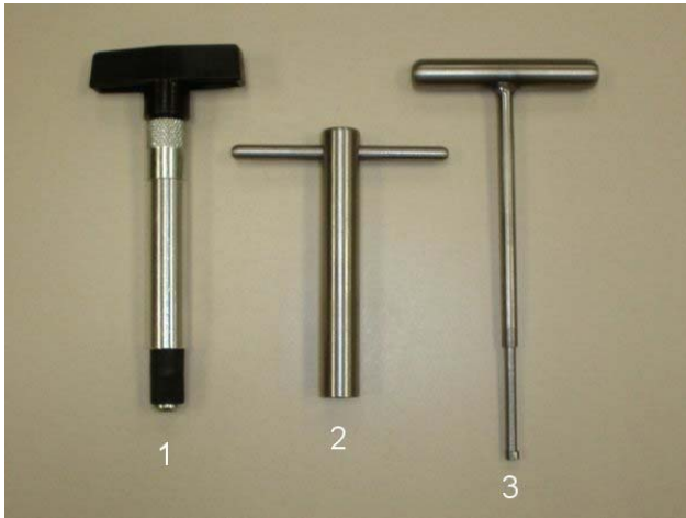
Figure 8 Crankcase-to-Head Tube Removal Tool
