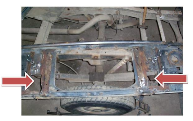
I started by removing the core support boxing just above the frame mount. I used a plasma-cutter to remove the unneeded boxing (much better than a torch, less heat). Don't forget to cut holes for the air ports to go through.
