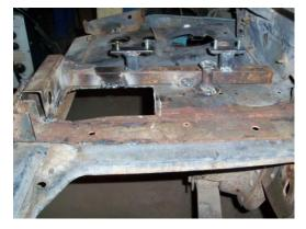
I attached a piece of 1"  $\times$  1" square tubing to add support for the boxing I removed. I also but the mounts on the tubing for the framing I constructed to hold the grill.
