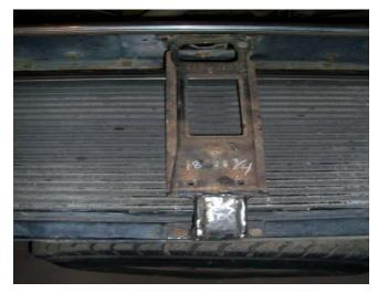
I didn't want to use pins on the hood so I took the hood support bracket and cut the bottom off of it and constructed a new base that would bolt into the original location. I used 3/16" x 1" strap to make it. I had the intercooler sitting in-place when I was fabricating so I could make I had proper clearance. I used my backup core support to get the measurement correct for the grill to sit properly in place.
