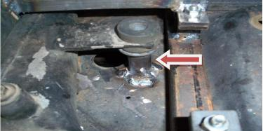
This is a little spacer I made using a piece of round tubing and a 1/2" flat washer welded on each end. I then used a  $\frac{1}{2}$ " x 4  $\frac{1}{2}$ " bolt to secure the top of the intercooler.
