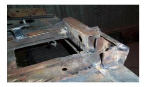
I took a piece of 1"x 2" tube and drilled a 1" hole in for the base of the intercooler to sit in. This sits right next to the bracket for the frame mount.
