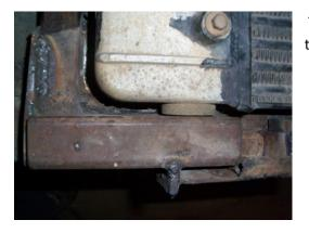
This picture shows the grommet of the base of the intercooler sitting in the 1" hole.
