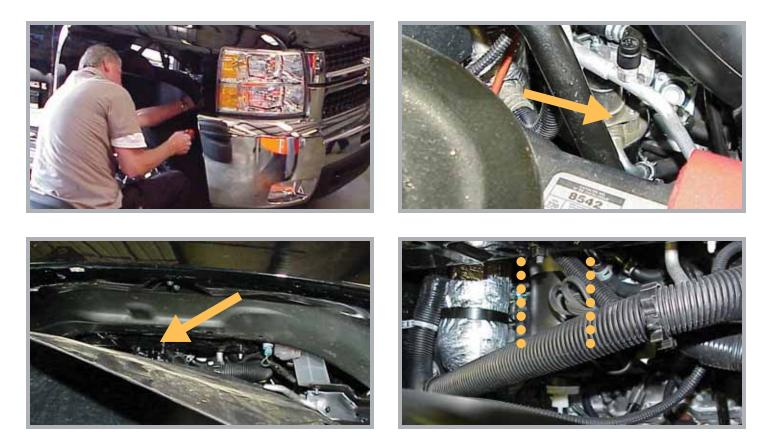
In addition to more durability and better performance, the upgraded design of the WIX 33960 offers the installer an easier installation and removal process. The tapered design of the filter shell provides for increased external clearance that eases the tight fit during installation and removal.
