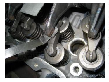
Use your .012" feeler gauge between the rocker arm and the valve bridge as pictured. The correct setting is had when there is slight resistance when moving the feeler gauge. It should not be so tight that the gauge can not be removed. Once the proper setting is made, tighten the jam nut while holding the adjustment screw. Verify that your setting has stayed after tightening the jam nut.
