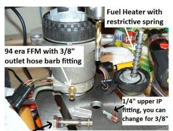
Lower IP fitting with 4 holes bored to 5/32" and screen that covers the holes. There is a screen on the bottom of the fitting too that should be cleaned.
