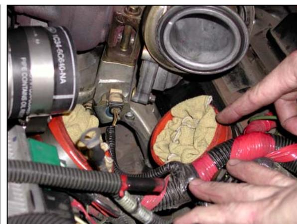
5. Loosen hose clamps and remove the x-section pipe from the engine. Cover intake manifold openings to prevent foreign objects from entering the pipework during this installation
