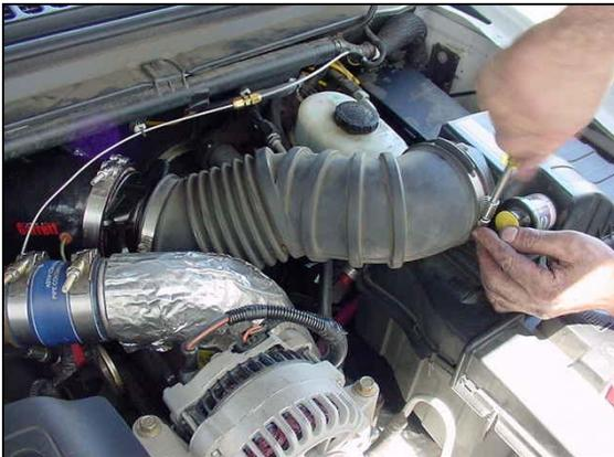
23. Re-install the hose from the breather duct to the air filter housing, snug the clamps. Reconnect battery, and you're DONE!!
