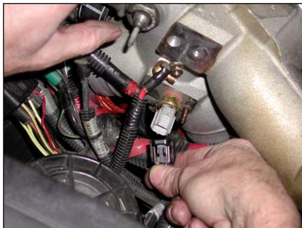
4. Unplug any remaining hoses and electrical connections from the x-section pipe
