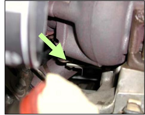
8. Reach under turbo and slide the clip on the EBPD control rod towards the pedestal to free the EBPD crank
