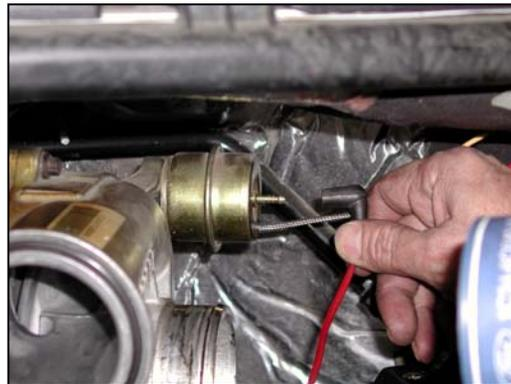
9. Remove the 2 bolts holding the turbo to the pedestal and unplug the red pressure line from the actuator
