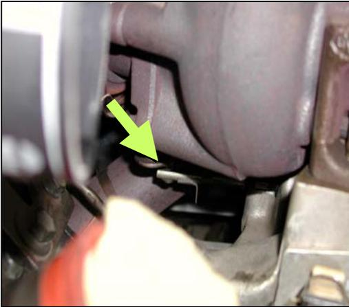
14. Ensure the crank pin for the EBPD drops into the hole in the control arm rod-end. Slide retaining clip back into place ensuring the clip fits into the crank pin groove.
