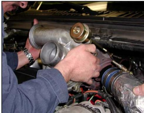
10. Make note of the turbo's position and how it fits on the engine for future reference. Lift the turbo off the pedestal and remove from the vehicle.
