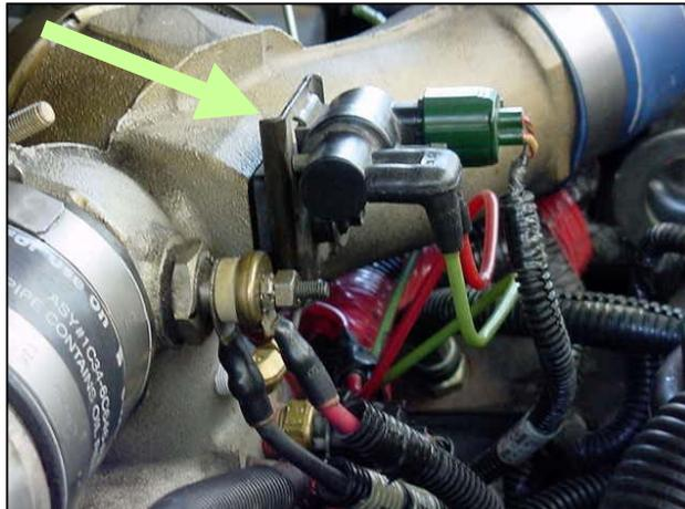
2. Remove the boost control module from the front of the x-section pipe
