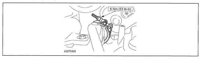
10. Make sure the exhaust inlet pipe is correctly aligned to the exhaust manifolds. Using hand tools, alternately tighten the nuts to draw the pipe to the exhaust manifold. There should be an equal gap spacing between the pipe flange and the exhaust manifold flange at the top and bottom bolts.
