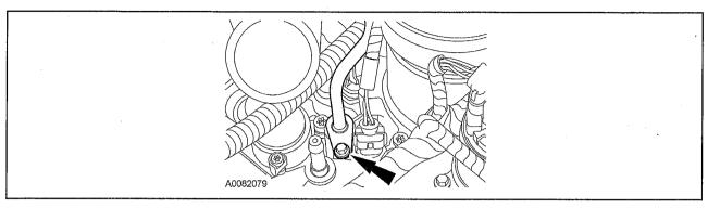
16. Remove the rear turbocharger mounting bolt.
