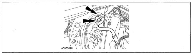
7. Remove the bolt and the wire retainer.
