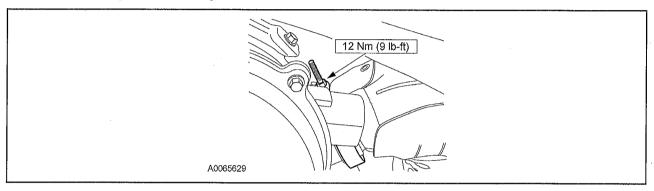
9. Position the clamp and tighten to specification.
