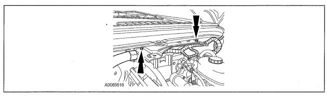
5. Disconnect the turbocharger variable vane hydraulic control valve electrical connector.
