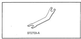
Disconnect Tool, Quick-Release Coupling 303-755
