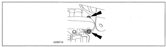
12. Loosen the RH exhaust inlet pipe-to-exhaust manfold nuts.
