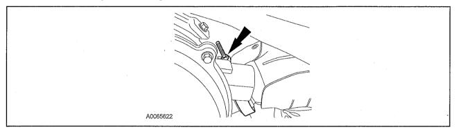
10. Loosen the exhaust inlet pipe-to-EGR cooler clamp.
