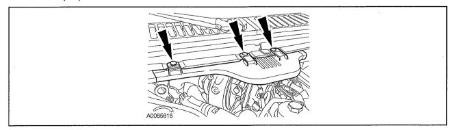
4. Disconnect the two wiring harness push pins and position aside.
