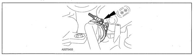
11. Loosen the LH exhaust inlet pipe-to-exhaust manifold nuts.
