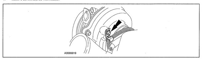
8. Remove the marmon clamp from the turbocharger outlet.
