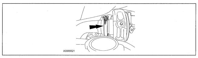
9. Remove the marmon clamp from the turbocharger inlet.
