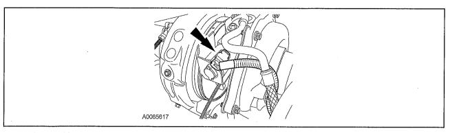
17. Position the wiring harness and connect the pushpins.
