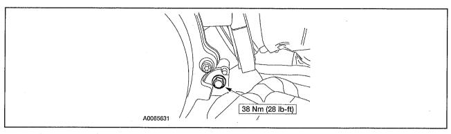
8. Install the turbocharger inlet marmon clamp.
