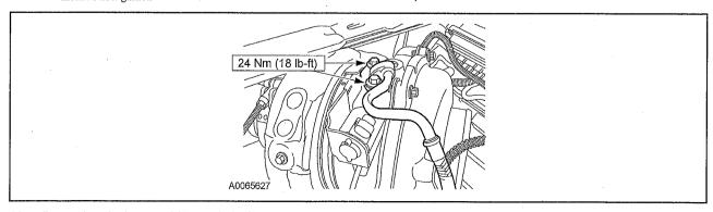
16. Connect the turbocharger variable vane hydraulic control valve electrical connector.
