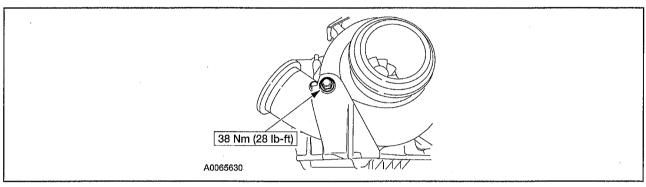
6. Install the oil feed tube.
