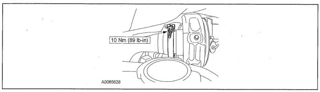
13. Position the wire retainer and install the bolt.
