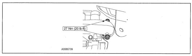
12. Install the turbocharger exhaust marmon clamp.
