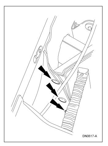
10. Remove the three air deflector pin-type retainers and the air temperature sensor.
