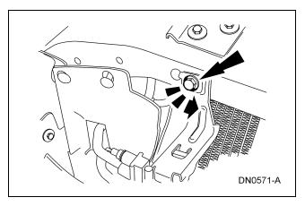
7. Unclip the hood release cable from the radiator support.
