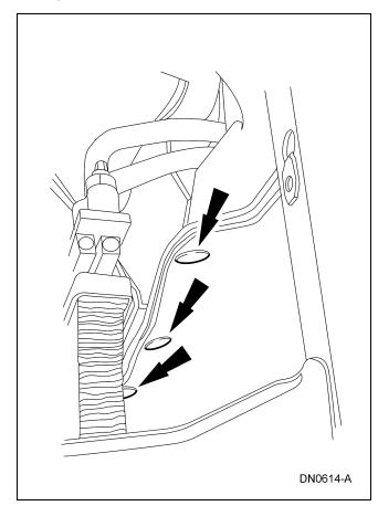
9. Remove the air deflector push pins from the left rear air deflector.
