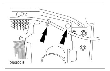
6. Remove the air conditioning condenser brackets.
