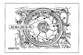
3. To install, reverse the removal procedure.
