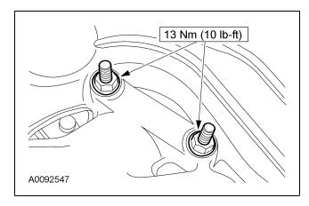
5. Install the intake manifold. For additional information, refer to Section 303-01C.
