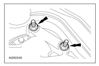
3. **NOTE:** Use care when removing the EGR cooler not to lose the grommets or spacer. Remove the bolt and the EGR cooler.
