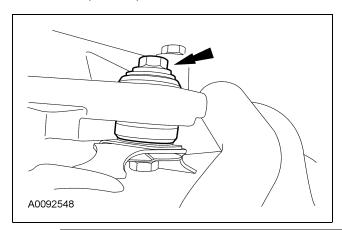
4. Tighten the EGR cooler stud bolts.
