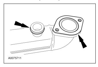
2. **NOTE:** Apply clean engine oil to the O-ring seal.
