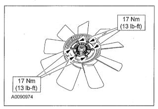
6. To install, reverse the removal procedure.
