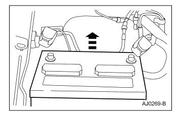
4. **CAUTION:** Be sure the battery cover is reinstalled to avoid premature battery failure.
