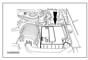
3. Remove the bolt and the battery hold down clamp.
