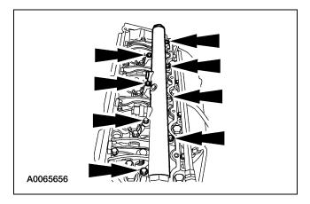
5. Disconnect and remove the high-pressure oil supply line.
