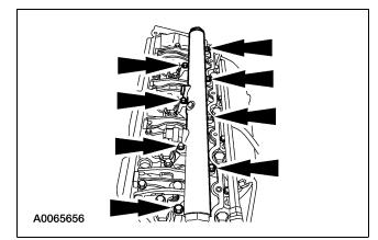
7. Tighten the bolts in the sequence shown.
