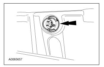
5. Apply engine oil to the top fuel injector O-ring seals.
