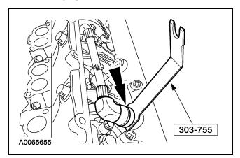
4. Remove the bolts and the high-pressure oil rail.
