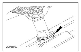
3. Disconnect the high-pressure oil rail supply line at the high-pressure oil rail.
