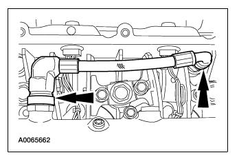
9. Connect the fuel injector electrical connector.
