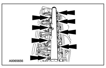
28. Tighten the bolts in the sequence shown.
