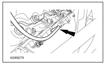
19. Remove the bolts and turbocharger heat shield.
