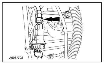
33. Install the fuel injection control module mounting bracket.
