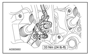
25. *NOTICE:* Make sure the injector wiring is clear of all moving parts or engine damage can occur.
