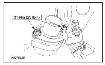
15. Tighten the exhaust backpressure tube fitting at the exhaust manifold.
