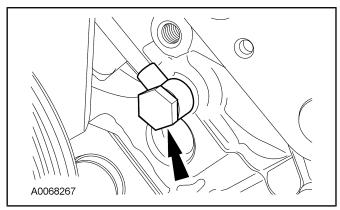
11. Install the fan shroud mounting stud.
