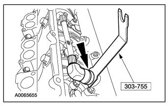
10. Remove the bolts and the high-pressure oil rail.
