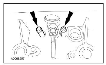
34. Remove the outer cylinder head bolts.
