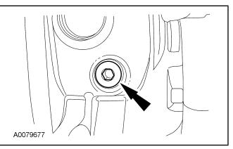
5. Remove the fuel injector control module mounting bracket.
