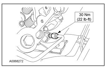
16. Position the fuel tubes and install the fuel tube bracket retaining bolt.
