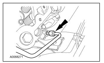
23. Remove the retaining nuts. Remove the exhaust back pressure sensor and tube assembly.
