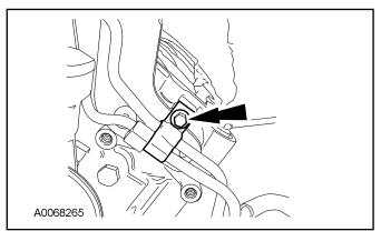
25. Remove the bolt and the idler pulley.
