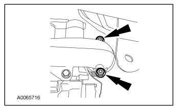
17. Remove the turbocharger adapter pipe.
