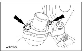
24. Remove the retaining nut from the fuel tube bracket and position the fuel tubes aside.
