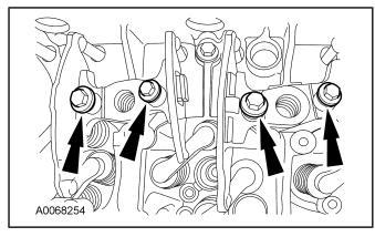
32. Mark the eight valve bridges with a permanent marker and remove.
