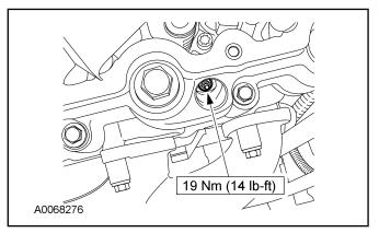
18. **NOTE:** Clean and apply clean engine oil to the O-rings before installing.
