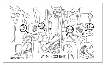
7. *NOTICE:* Using too much engine oil on the threads of the cylinder head bolts can cause damage to the threads and poor sealing. Using anti-seize compounds, grease or any other lubricants other than engine oil on the cylinder head bolt threads can affect the true torque value of the bolts.
