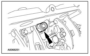
30. *NOTICE:* Make sure the insulation blanket is not damaged (torn, cracked or fabric separated from the metallic skin) when removing the lower rear cylinder head bolt. If the insulation blanket is damaged, the entire blanket must be replaced.
