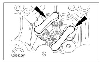
33. *NOTICE:* To prevent engine damage, keep the push rods in the order in which they were removed. Install all push rods back in their original positions.
