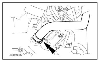
27. Remove the fan shroud mounting stud.
