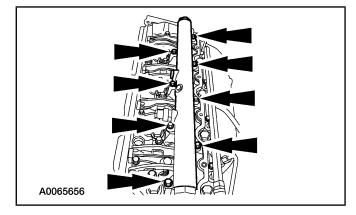
11. Disconnect and remove the high-pressure oil supply line.
