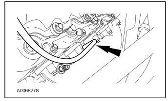
20. Install the turbocharger heat shield and bolts.
