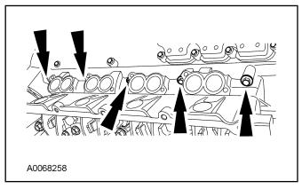
4. *NOTICE:* To prevent engine damage, keep the push rods in the order in which they were removed. Install all push rods back in their original positions.
