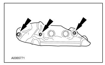
20. Remove the glow plug buss bar.
