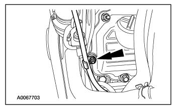
8. **NOTE:** Mark the position of the valve cover bolts for valve cover bolt installation.
