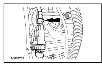
7. Remove the nut and position the oil level indicator and tube aside.
