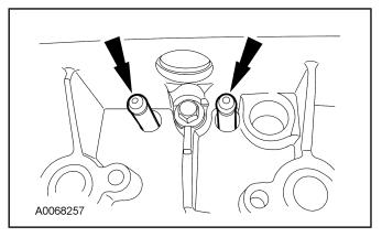
5. **NOTE:** Coat the end of each valve stem with clean engine oil.
