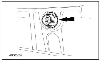
26. Apply engine oil to the top fuel injector O-rings.
