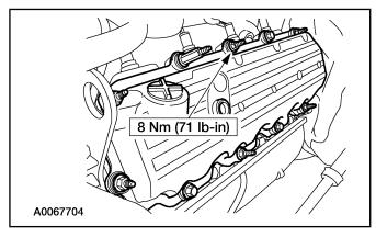
31. Position back the oil level indicator and install the nut.
