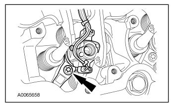
15. **NOTE:** If a snap ring or a piece of a snap ring is missing from the injector hold-down assembly, it must be located prior to removing the shop towels.
