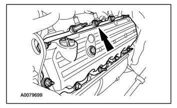
9. Disconnect the high-pressure oil rail supply line at the high-pressure oil rail.
