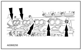
35. Install the special tool and the lifting crane. With the help of an assistant, remove the cylinder from the vehicle.
