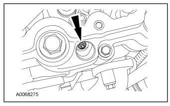
22. Disconnect the exhaust back pressure tube at the exhaust manifold.
