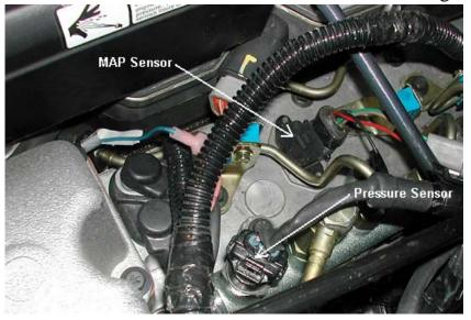
pressure sensor connector into the stock pressure sensor on the engine and the stock engine wiring harness connector into the supplied pressure sensor connector.
