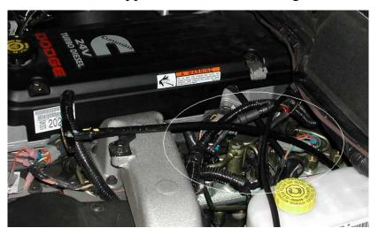
harness in the engine compartment. Disconnect the stock wiring harness at the MAP sensor located on top of the intake manifold. Plug the supplied MAP sensor
