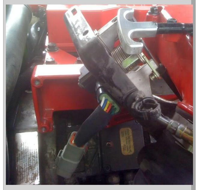
The paperclip goes into the number 3 wire. Gently press the paperclip pass wire until it makes contact with the connector.
