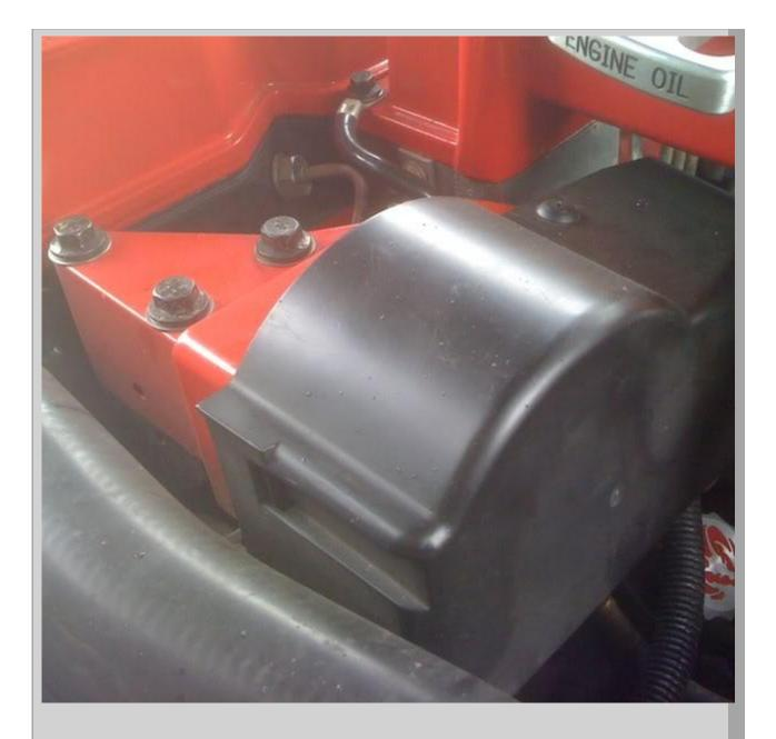
There are 2 plastic screws that hold the cover in place. One is easily visible at the top of the cover, the other is at the front of the cover under the radiator hose. You can see the second screw here:
