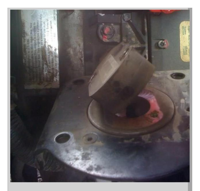
Disconnect the electrical connector from the factory APPS, and carefully install the new Williams APPS:
