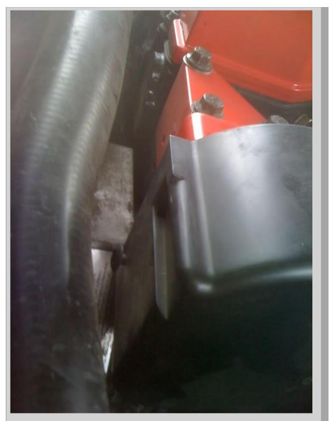
The screws are the standard Phillips screw, but they hold a small plastic tab through the cover and into the metal APPS holder. This picture should give you an idea of how the
