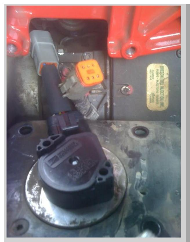
The kit comes with new screws that use a standard Phillips head bolt instead of the torx head. Instead, I decided to reuse the factory torx bolts. As you install the sensor, be
