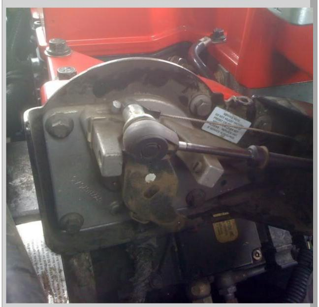
Remove these bolts, but do not remove the cables!
