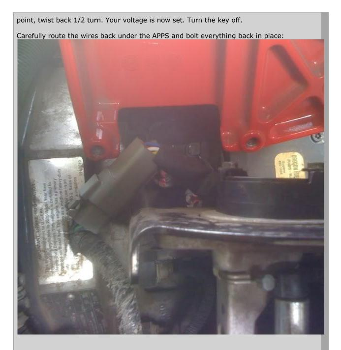
Turn the key back to the on position, and slowly depress the pedal to the floor and slowly allow it to return to the idle position. Turn key off. Turn key back on and slowly depress and allow pedal to return again. Turn key off.
