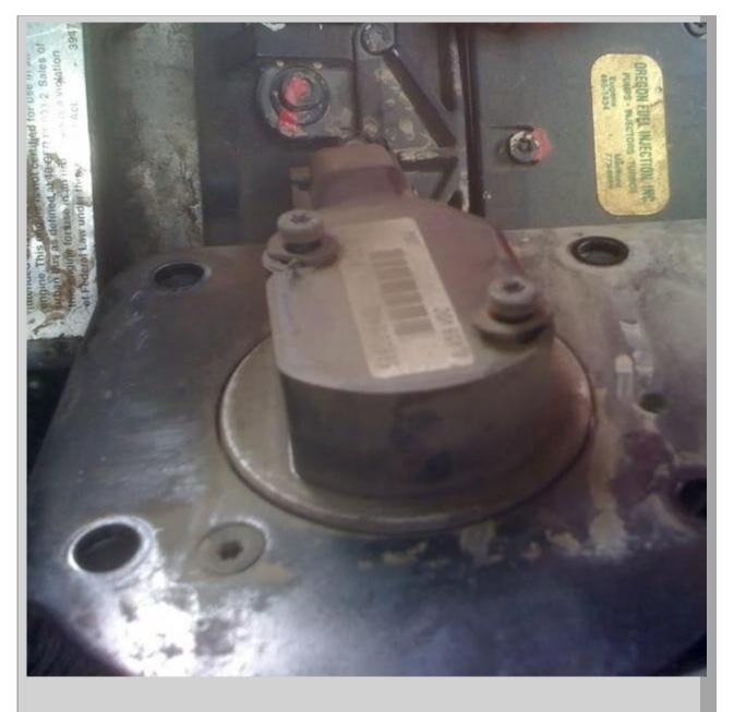
Remove these 2 screws and you can remove the factory APPS:
