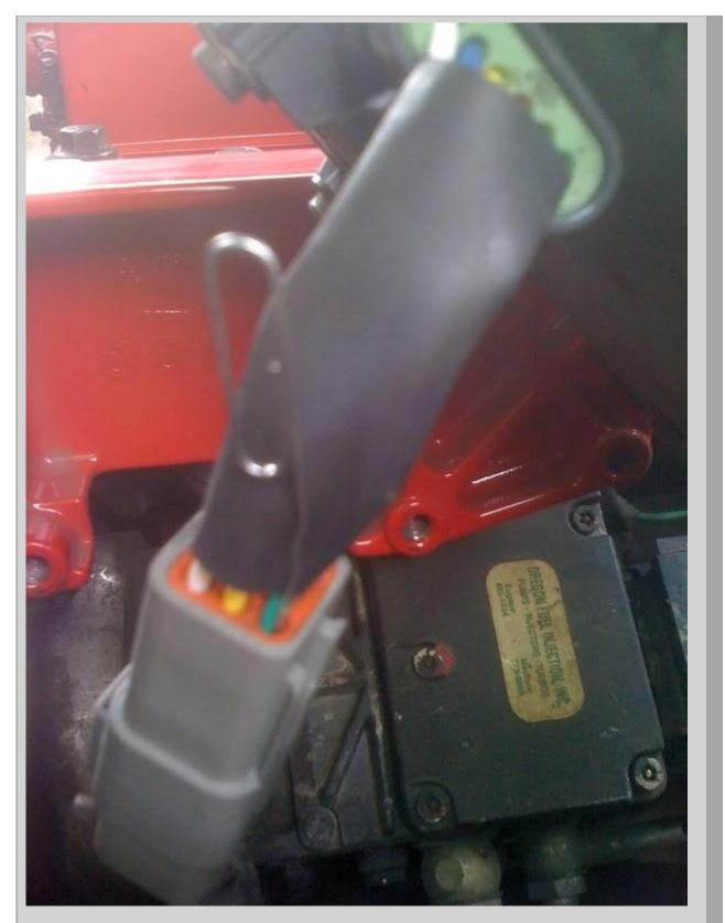
Reconnect the batteries, and turn the key to the on position. Use a multimeter to check the voltage of the new APPS. The instructions come with an acceptable range, and mine
