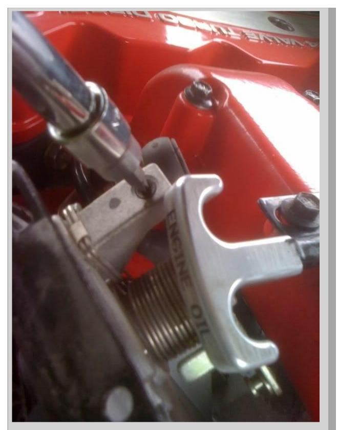
You tighten the bolt until the voltage just begins to rise. Mine took several turns before the voltage on the multimeter changed.
