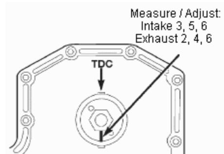
(8) With the engine in this position (pump gear mark at 6 o'clock), valve lash can be measured at the remaining rocker arms:
