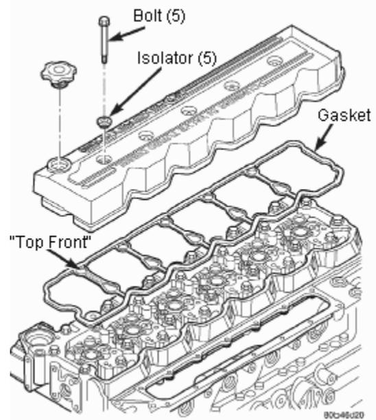
Clean and inspect the cover gasket and isolators, they are reusable if they are not cracked.
