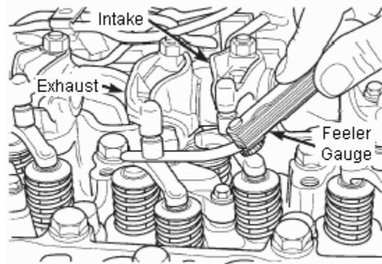
Acceptable Intake lash range: 0.006 in. (0.152 mm) to 0.015 in. (0.381 mm)
