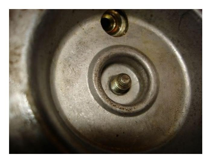
To adjust smoke screw loosen lock nut 10mm, use 3mm allen wrench to adjust smoke screw in or out.
