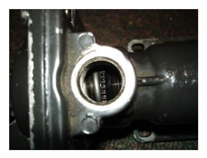
The best way to adjust the starwheel for proper fueling is to use regulated air. Use an air blow gun with a rubber tip, set pressure on compressor to the psi you want full fuel. I'll use 40 psi as an example.
