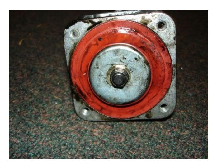
Next remove 10mm nut holding diaphragm on.
