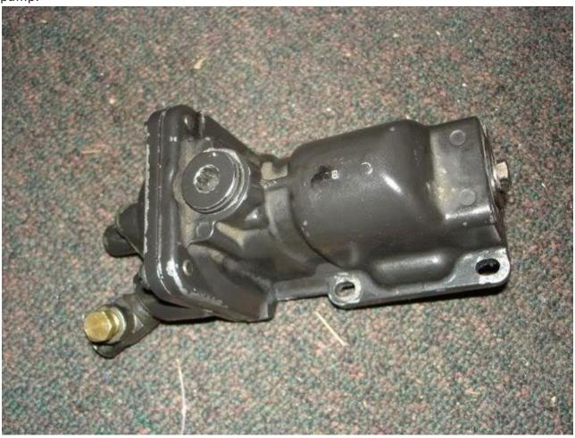
Next remove 4 screws (1 is a break off screw) to get to the afc diaphragm.
