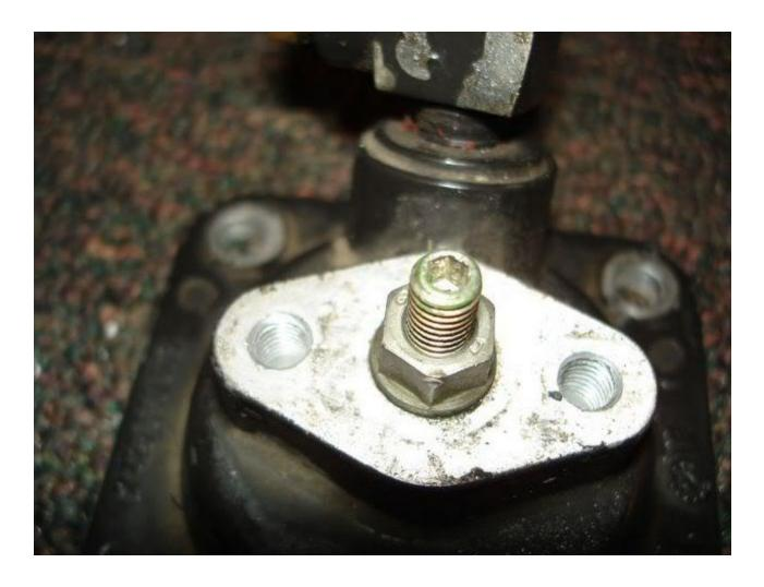
This controls the 0 boost fueling, the further in the screw the more tension it puts on the afc spring, allowing more fuel to come on with no boost.
