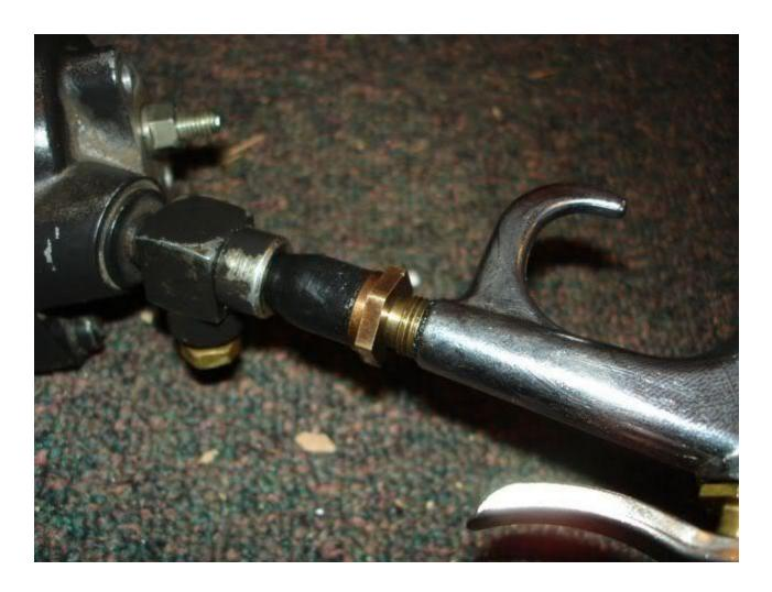
Adjust starwheel until afc foot travels completely forward with 40 psi of air. The more tension thats on the spring the more psi needed to move the foot forward. Too much tension on the spring will cause the spring to bind up and the foot will not move all the way forward.
