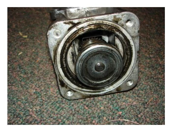
Once the diaphragm is off remove the cupped washer on the spring side and replace it with a flat automotive body washer with the same outside diameter and 8mm hole.
