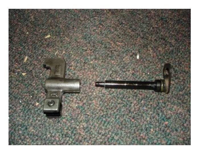
Now grind 1/16" to 1/8" off the round part of afc foot that slides on the shaft.
