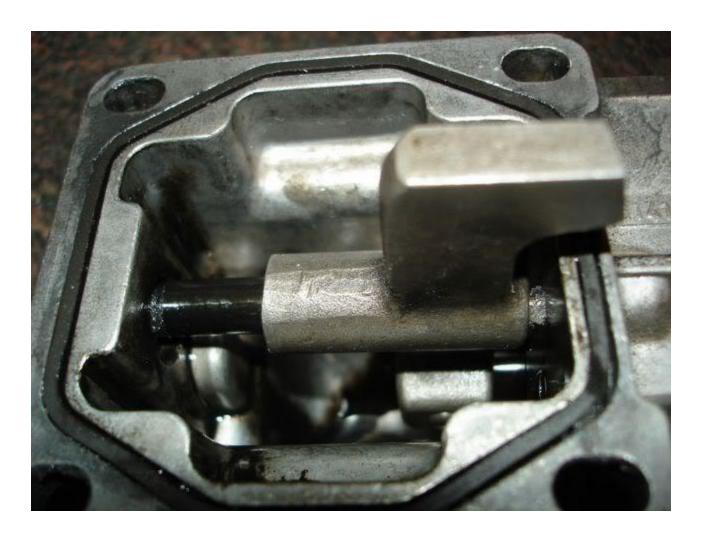
Install starwheel plug back on afc.
