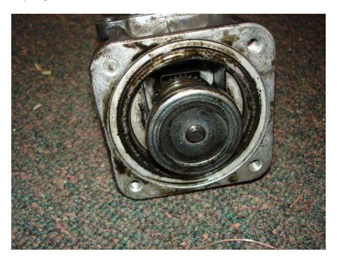
Remove the cupped washers and grind them flat OR replace them with fender washers from the local hardware. I have found a  $1\,\%''$  diameter outside and 5/16'' hole washer fit fine and can be purchased for under a \$1 a piece.
