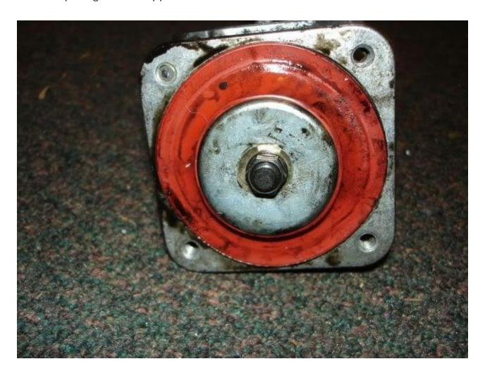
Remove the 10mm nut holding the Diaphragm to the AFC shaft. There should be another slightly cupped washer under the diaphragm.
