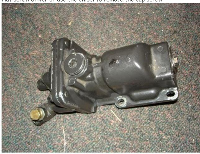
Now you can remove the 4 screws on the back of the housing to reveal the AFC Diaphragm. One of these is a break off/Tamper proof cap screw as well.
