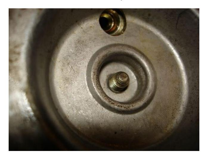
Smoke screw adjusted all the way out.
