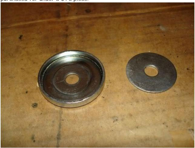
Now that the washers are replaced you can put the diaphragm and cover back on.
