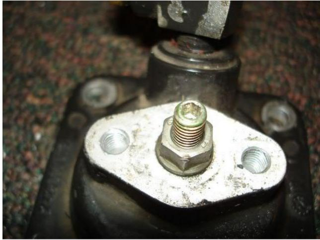
This screw controls the O/No boost fueling. It pushes on the end of the AFC Diaphragm and pushes the foot forward for more rack travel at no boost conditions. This can be adjusted at anytime and you can set it to your likening. To adjust smoke screw; loosen the lock nut (10mm), use 3mm allen wrench to adjust screw in or out.
