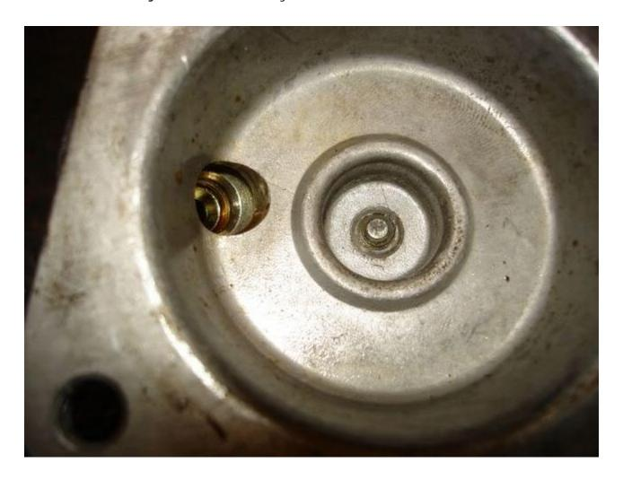
I start out with the screw just touching the diaphragm and then tighten it up from there. You should be able to feel the screw touch the Diaphragm as you will get some resistance from the AFC spring.
