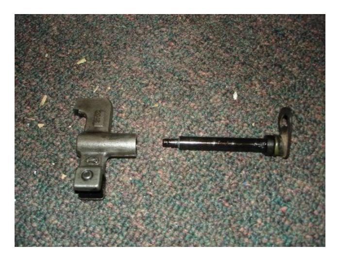
Measure the barrel of the foot and mark 1/16" to 1/8" and grind that off the REAR of the barrel. This will allow the AFC foot to travel past the plate when set FF so you can get full rack travel.
