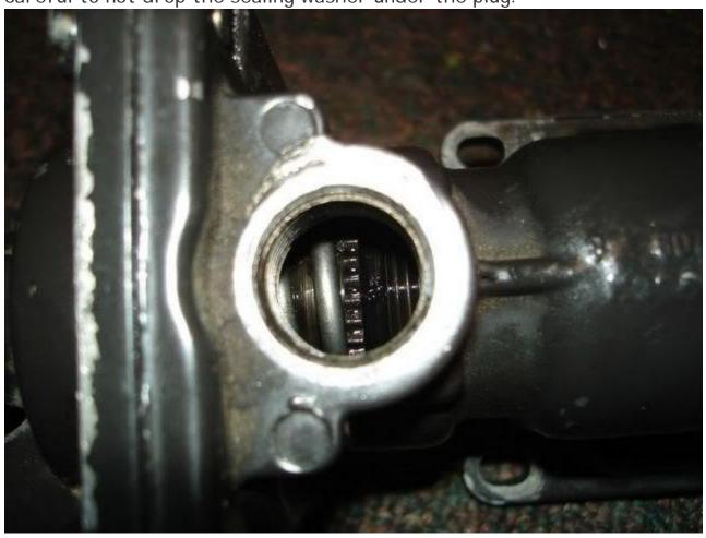
The best way I have found to get the initial adjustment for the starwheel is to use regulated compressed air. Get a blow gun with a rubber tip and put the tip where the boost reference line to the AFC comes in at.
