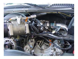
d) Sensor is directly behind A/C compressor under rigid coolant and should be easy to access. Do not connect to similar sensor which is located to the right of the boost sensor. It is called the Barometric Sensor and looks identical as the boost sensor
