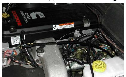
main wiring harness in the engine compartment. Disconnect the stock wiring harness at the boost sensor located on top of the intake manifold. Plug the supplied MAP sensor connector into the stock engine
