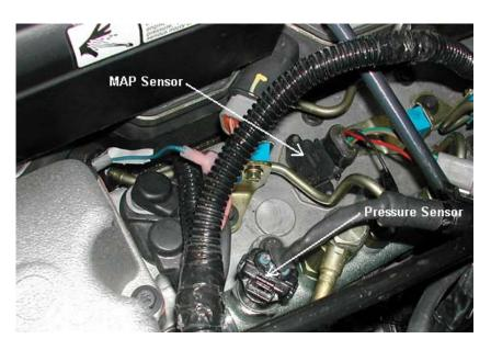
supplied main wiring harness in the engine compartment. Disconnect the stock wiring harness at the sensor located on the main fuel rail on the driver's side towards the rear of the engine. Plug the supplied
