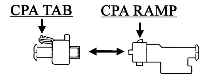
NOTE: Illustration shows correct orientation on connector
