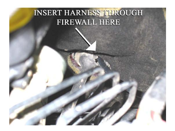
Route the module connector up to where the module will be mounted. Make sure to not route the wires near the brake, clutch or gas pedals or any movable parts on the steering column. Loosen the screws on the back of the module approximately three turns. Plug in the Striker harness to the module and tighten the screws. Use the supplied Velcro strips and attach the module permanently.
