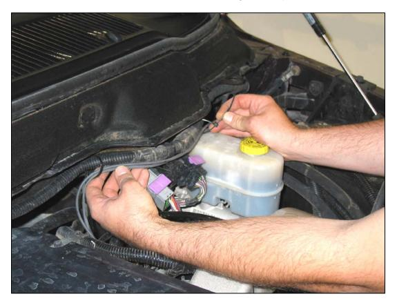
Locate a good place to route the Striker harness through the firewall of the truck and into the cab area. This rubber plug is an ideal place to do so. If the truck has a 6-speed transmission, make sure to not route the wires where the clutch pedal will rub on them.
