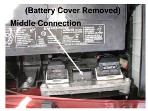
5. Insert the other end of the EZ wiring harness to the middle connector on the PCM.
