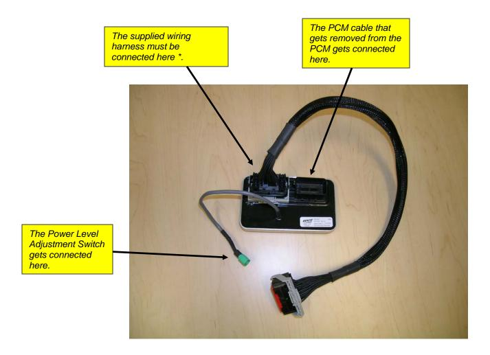
\*Note: If the PCM cable is not installed correctly, the truck will either run at the stock power level or not start (depending on the manufacture date of the truck). If either of these symptoms occurs, be sure and check your cable connections.
