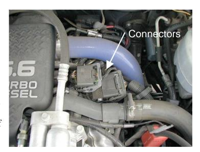
Notice: Use caution when inserting connector bodies. If the connector does not slide smoothly, remove the connector, inspect the pins, and retry installation.
