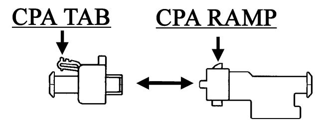
NOTE: Illustration shows correct orientation of connector latch
