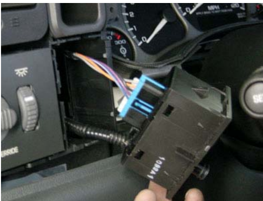
7. Feed wires into dash, re-attach connector, and snap power controller unit in dash. Assemble clasp, shift into P, and do not turn key on until complete.
