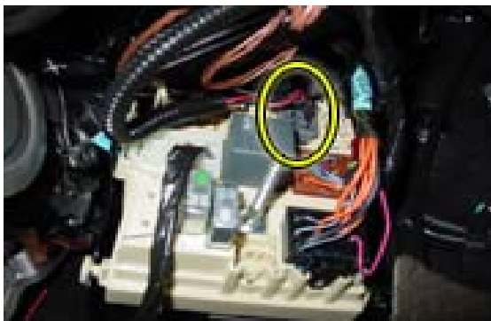
28. For 2003 & 2004 the six pin female socket is located on the top two sockets from the right. The image above shows the gray socket inserted in the proper location.
