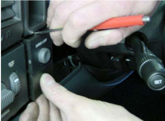
6. Trucks without Fog Lamps: Unlatch the retaining tab of the cargo lamp unit at the bottom first, then at the top, and remove.
