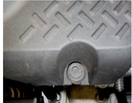
9. 2001 models: remove cover retaining bolt, or push forward on cover to release from rubber grommet.
