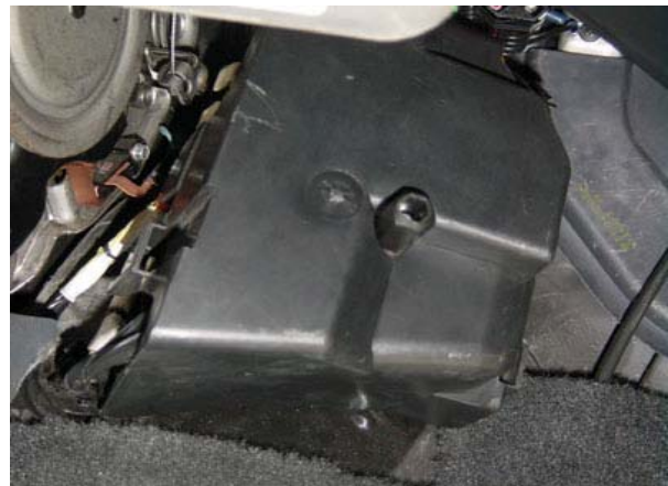
26. Remove the junction box cover located to the left of brake pedal, under the dash.
