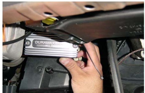
30. Mount the ECU under the dash to main GM harness behind aluminum support bracket with plastic tie straps.
