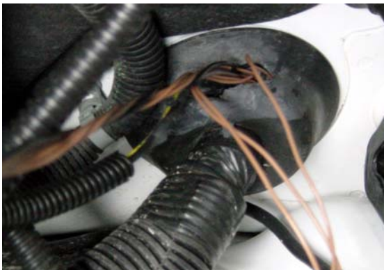
23. Tape the wire pairs one after another onto a coat hanger to protect the connectors from being pulled off the wire. Pass through the grommet to follow the existing wire bundle. The wires should be able to pass easily.
